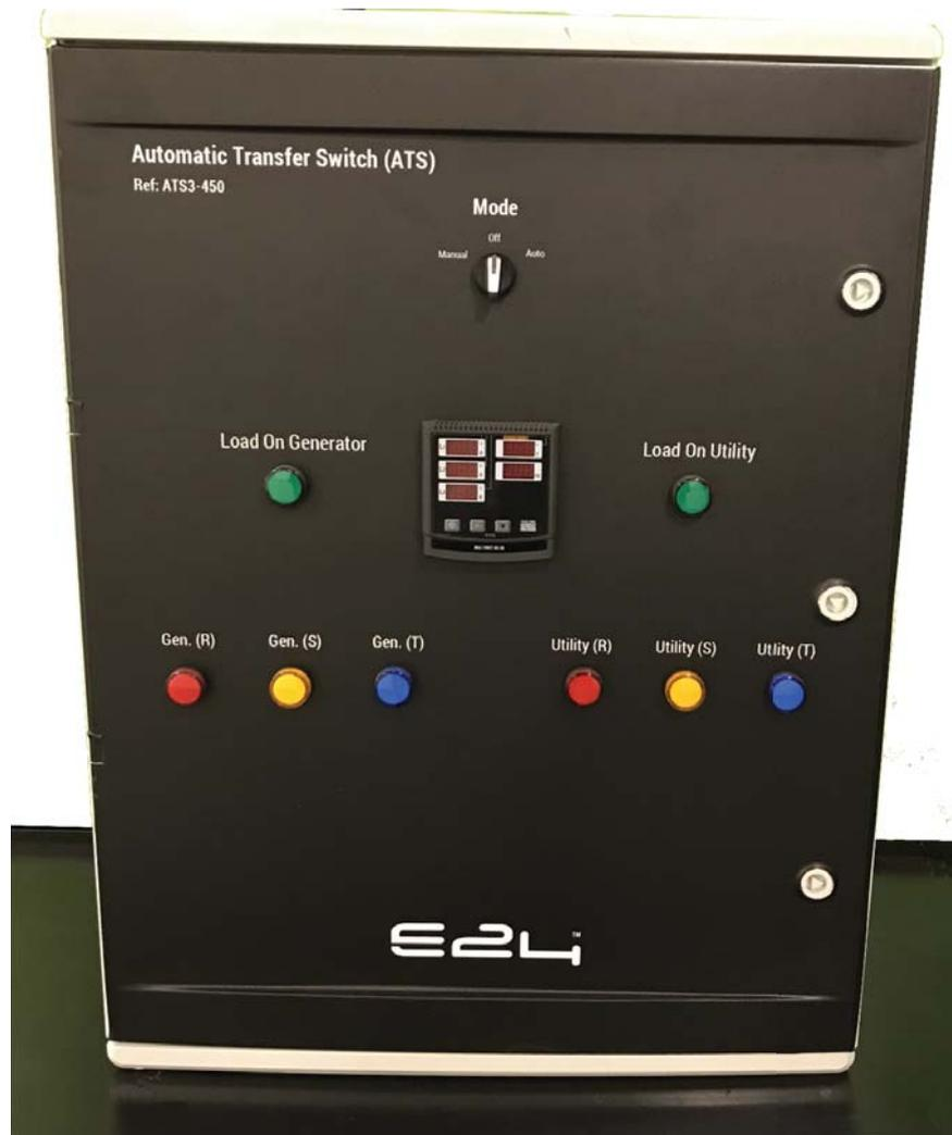
Automatic Transfer Switch Panels (ATS) are mainly electrical switches that switch the load between two sources. It is used when the client has a backup diesel generator and wants to integrate it with E24's Energy Storage System (ESS). ATSS supplies the input of the ESS and switches it between utility and diesel generator.
